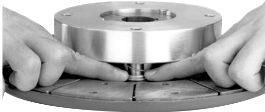
Figure 19 - Positioning the detent cups in the armature
