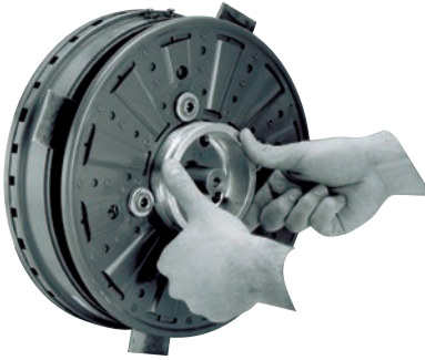
Figure 17 - Setting the airgap.
