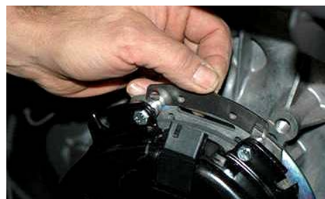
Brake shim can quickly be removed from clutch while mounted and the airgap can be checked easily.
