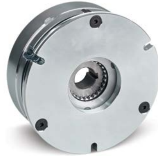
The PK (Very Thin) range is a pre-assembled on/off dry spring applied electromagnetic brake used for parking and emergency as well as some service braking.
