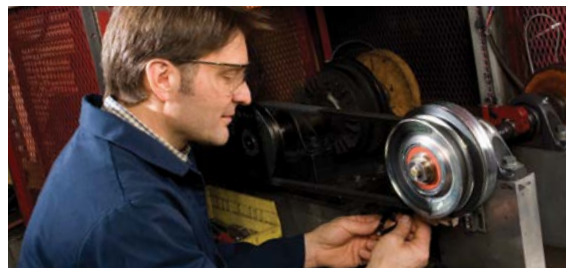
In-house inertia test stands feature belt-driven motors that allow zero-hour prototype brake and clutch torque testing.
