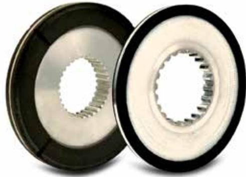
The friction disc on the left is for a unit designed for primarily holding only applications. The disc on the right, with a significantly greater amount of friction material, is for a brake designed for occasional stop cycling. The increased amount of friction material provides higher total cycle life.
